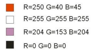
If we allow one byte for each of the three components, we can specify more than 16 million different combinations. This is actually more than the human visual system can distinguish.
